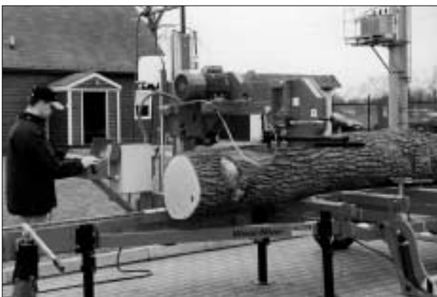
New sawmill range at Ligna will feature this enhanced version of Wood-Mizer's small LT15 with the addition of standard powerfeed up and down and optional manual hydraulic log loading.
