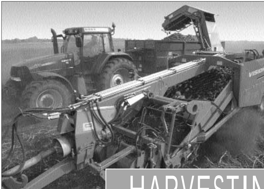
Standen Vision potato harvester and light cable connections to the tractor bottom left
