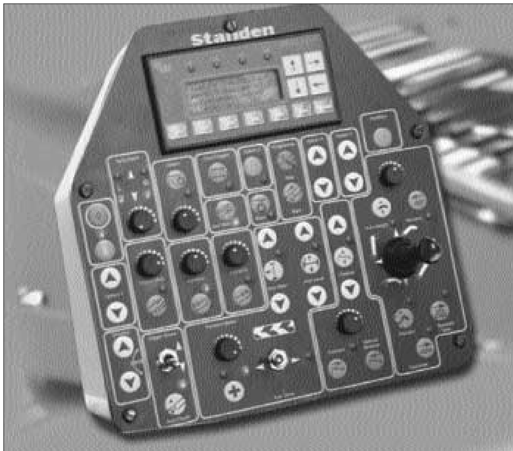
Driver Interface control unit for the Stander Vision harvester
