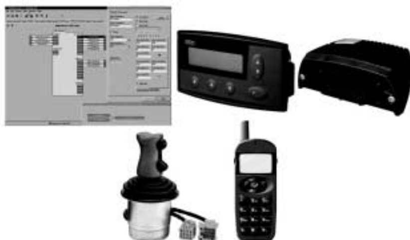
Hardware required for high complexity machines; IQAN master controller and various Controller Area Network (CAN) nodes
