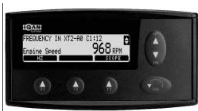
Example of a master module screen display reading engine speed; note hardware module location, hardware pin number and the speed as scaled value (option to display the Hz value also available)
