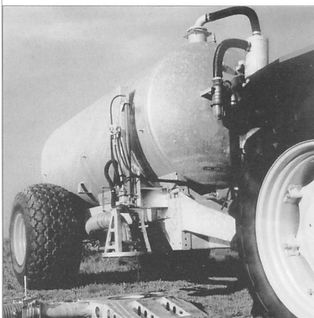
The Fast-Fill is a remote slurry tanker filling system. It has been developed to help reduce the time that is taken to fill a vacuum slurry tanker.
