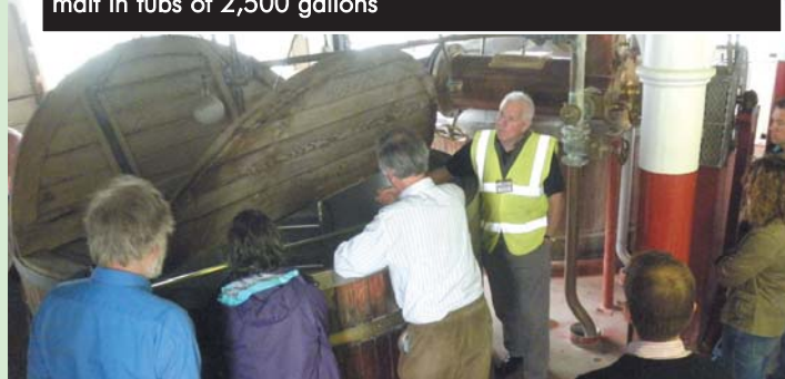
BELOW: The first stage in the brewing is the mashing of the malt in tubs of 2,500 gallons
