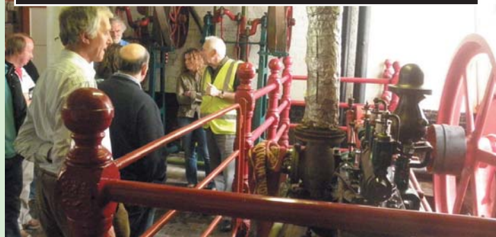
BELOW: The horizontal engine that still has the potential of driving the mill 'line-shaft' driven tower brewery
