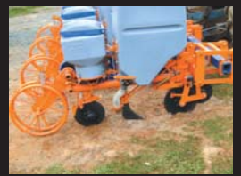
Figure 5. A low-cost no-till planter from Brazil (Knapik). The front vertical disc cuts through the mulch and is followed by a chisel-tined fertilizer applicator and a twin offset disc seed slot opener. Offset discs are generally preferred in high residue situations (>4 t/ha).
