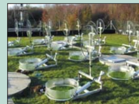
Figure 2. Gas flux chambers fitted to the lysimeters with lids open. The lids are closed in turn for gas flux measurements with air circulated through them to an isotope mass spectrometer in the instrument building.
