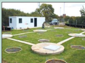
Fig. 1. The Wolfson laboratory prior to the installation of the gas flux chambers showing the instrumentation building, the buried lysimeters and manholes containing connections to the lysimeters, gas lines and control systems.
