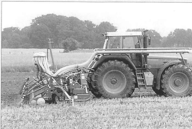
The front tanks are based on a 1500 litre – extendable to 2000 or 2300 litre – with a hydraulic fan to meter the seed of to the rear seed rail and an ability to handle either seed or fertiliser
