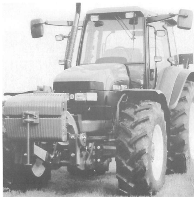
Lynx Front Linkages for New Holland TM Supersteer Tractors – Pictured is the new 3.5T Diamond SuperSteer front linkage from Lynx Engineering. The linkage is now available to fit 78.75 kW to 120 kW New Holland Series TM SuperSteer tractors. Tractors that are fitted with SuperSteer have a 65 degree turn angle which allows increased flexibility and manoeuvrability.
