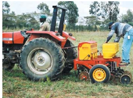
Figure 2. Direct planting with a Brazilian planter on a smallholder farm in Kenya
