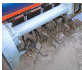
FIGURE 7. Chinese BG-6A full width, full cultivation one-pass seeder. Not CA. Photo: Brian Sims
