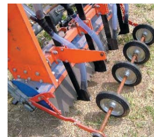
FIGURE 9. VMP seed and fertilizer delivery from an ACIAR-Rogro set up. Photo: Brian Sims
