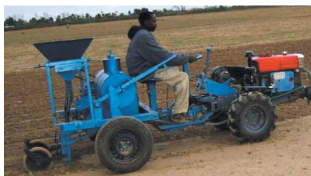
FIGURE 4. Ndume no-till planter and sprayer mounted on a Kungfu 2WT. Photo: Brian Sims.
