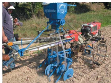
FIGURE 6. Thai Department of agriculture designed no-till drill for dry direct seeding of rice. Photo: Jack Desbiolles.
