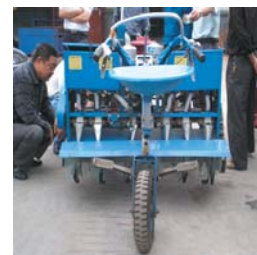
FIGURE 8. Full width rotary seeder / fertilizer modified for strip till sowing. Photo: Ken Sayre.
