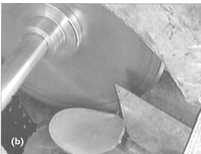
Fig.5. (a) Mango cheeks being cut from the stone passing between the two discs; and (b) position of one cheek after the cutting operation is complete
