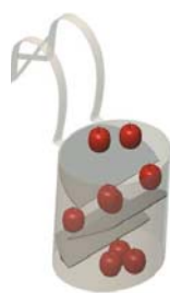
Fig. 7: Energy absorbing flaps for increasing picking speeds without bruising fruit
