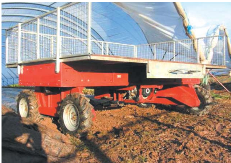
Fig. 27: Pik-King 1 motorized tray transporter
