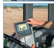
Figure 1. Upper image, a cluttered cab containing various terminals. Lower image, an ISOBUS virtual terminal
