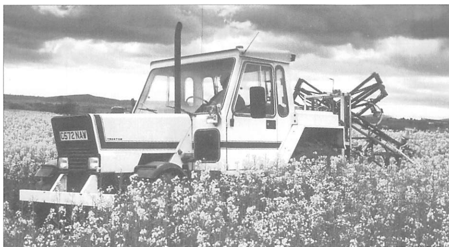
The lighter weight 4WD Trantor 'transport-first' tractor just completing work in the field and returning to the water source at speeds far in excess of that possible with 'ploughing-first' tractors.
