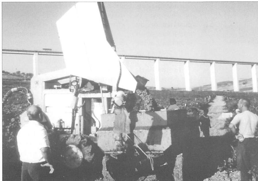
Fig. 5 Hopper unloading the harvested grapes into a trailer
