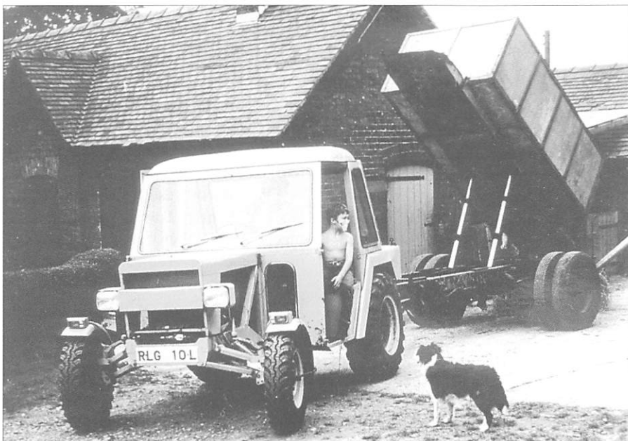
The prototype 41 kW Trantor at harvest time in 1973; designed to pull a bigger trailer than a Land Rover but travel at Land Rover road speeds
