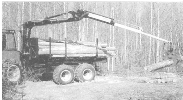
The new 10 tonne capacity Cranab 720 is fitted with the same slewing motor as the 8 tonne-metre crane, giving it greater power
