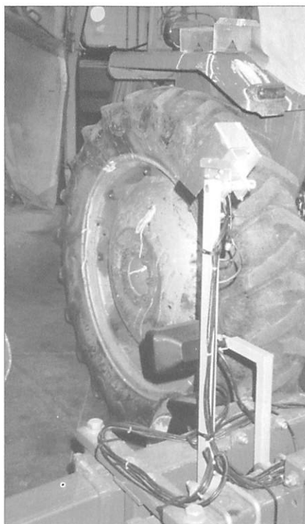
The simple video camera, which 'looks' at a row of plants, is seen here mounted on the frame of the hoe which it keeps in line irrespective of the tractor's position.
