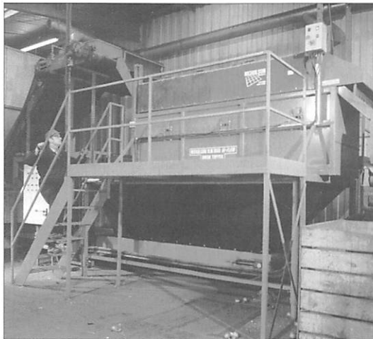
Nicholson Machinery's new high capacity onion topper is designed to work straight from store and produce onions to exacting retail standards, quickly
