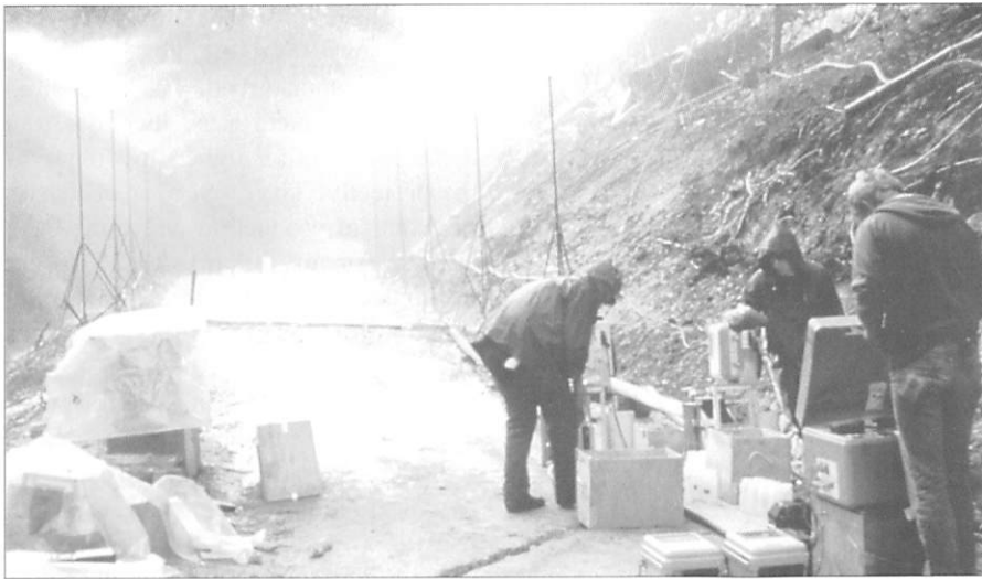
Fig. 1 Measuring road erosion rates in central Idaho with a rainfall simulator
