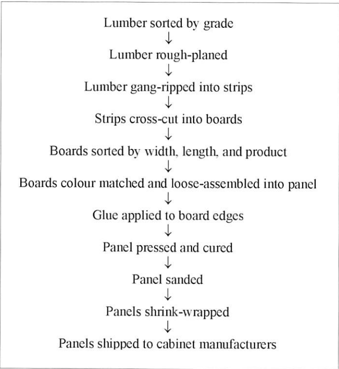
Fig. 8 Typical manufacturing process of edge-glued panels (Phelps et al., 1994)
