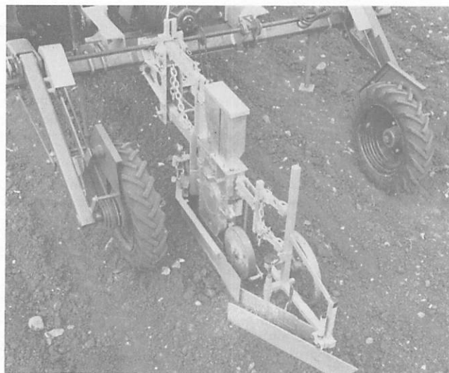
The NIAE prototype high-speed precision drill (courtesy NIAE)
