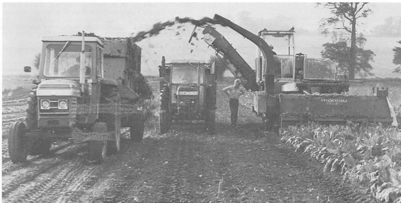
Harvesting both roots and tops from 6 rows at a time with the Moreau AT64 on J D Alston's farm at Kenninghall, Norfolk
