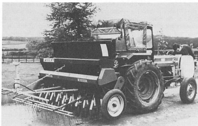
Experimental low volume spray bar attachment fitted to the rear of a standard corn drill
