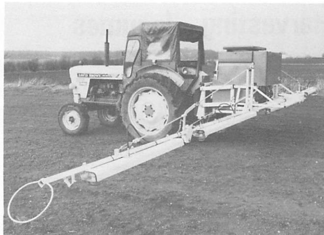
Commercial controlled droplet application sprayer (copyright Horstine Farmery Ltd)
