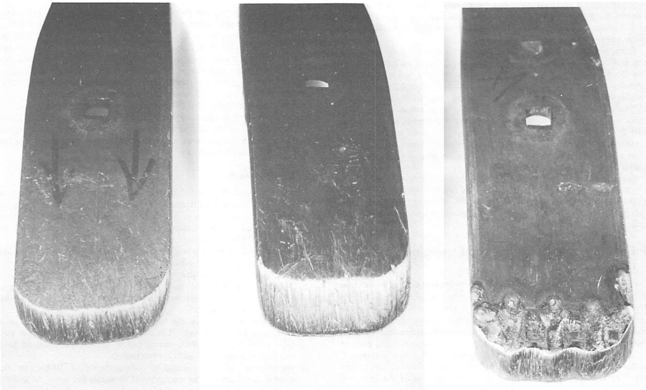
Fig 4 Comparison of wear 'land' on the underside of chisel plough points
