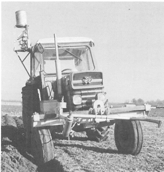
Fig 6 NIAE optical furrow-follower for automatic ploughing.
