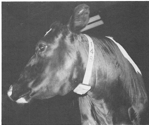
Fig 4 NIAE automatic identification unit for cows, mounted on a standard collar.
