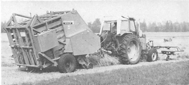
Fig 5. Experimental system for combined preservative application, windrowing and baling.
