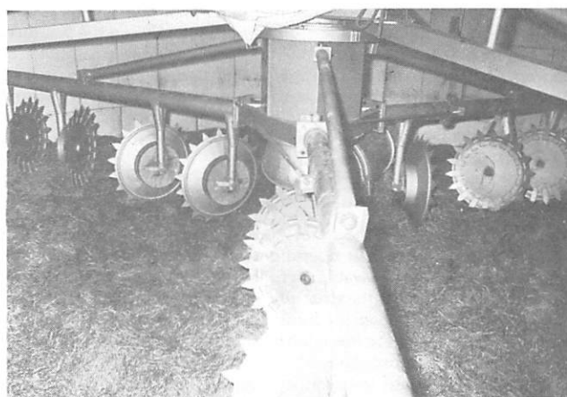
Fig 4. (below) The top unloader for long ensilage. The suction pipe of the blower is shown in the centre.
