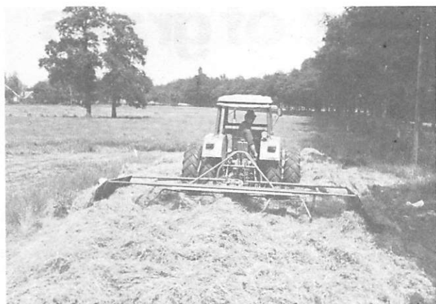
Fig 2. Rotary spreader mounted on the tractor used to consolidate the ensilage. Handwork at the clamp is eliminated.
