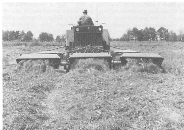
Fig. 1. The 4.8 m mower in front and three conditioners on another three point linkage in the rear.
