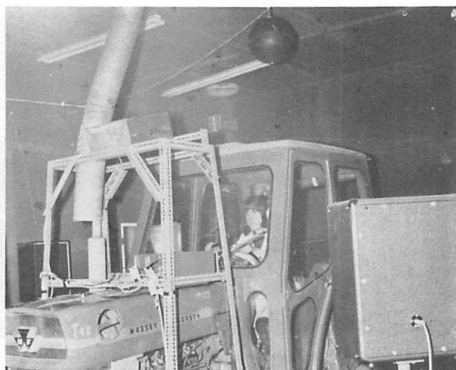
Fig 8 Tractor with simulated driving task in noise chamber to study the perception of sounds external to the tractor.
