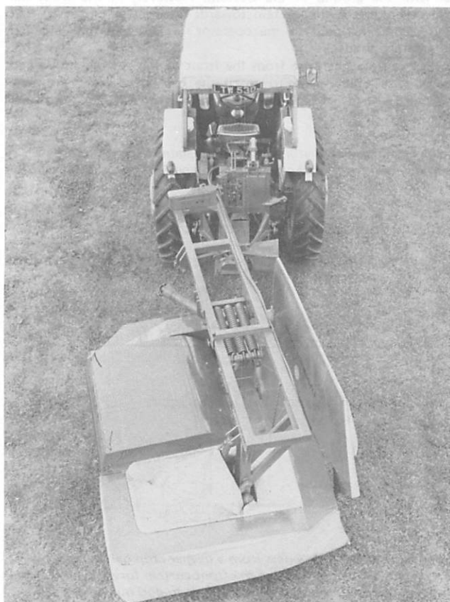
Fig 6 NIAE experimental mower-conditioner in transport position with extended front cover raised and locked.
