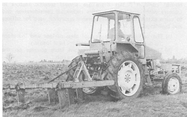
Fig 9 Tractor fitted with NIAE experimental suspended cab.
