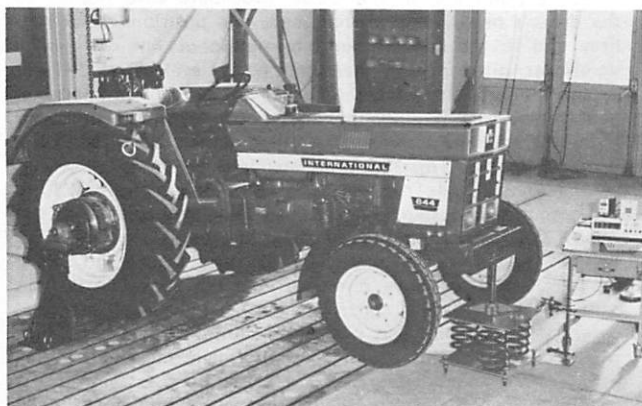
Fig 3 Arrangement of pivots and springs for tractor pitch, moment of inertia determination.
