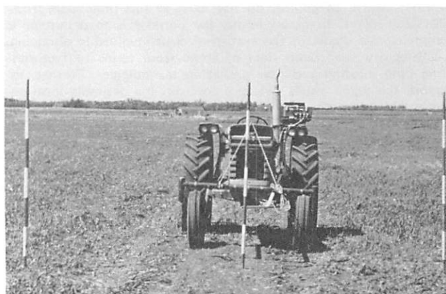
A driverless tractor on test at University of Saskatchewan, during IFAC Conference, June 1974. Tractor is back on the centre line after completing a circuit.
