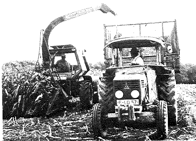
Fig 18 Intrac 2005 with front-mounted 2-row maize forage harvester.
