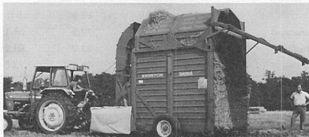
Fig 3 The Hesston Stackhand stack builder about to deposit a stack.
