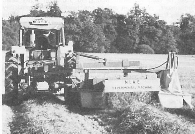
Fig 1(a) Two drum 2.13 m (7 ft) experimental semi-mounted mower — conditioner developed at NIAE, general view of machine at work showing swath.
