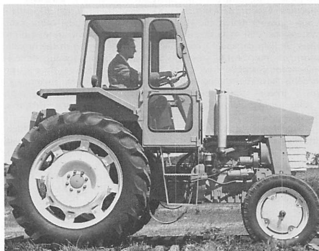
Tractor fitted with experimental suspension cab for ride improvement.
