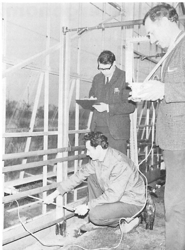
Measurement of airflow in a fan ventilated glasshouse.
