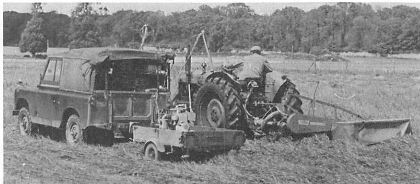
Field measurements of the performance of a rotary mower.
