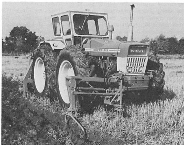
Fig 3 General view of device fitted to tractor with hydrostatic steering.
