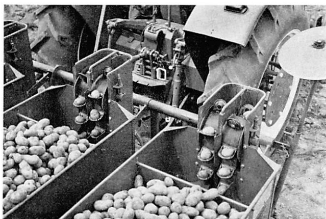
Fig. 3 (above) Automatic planters with two chains
