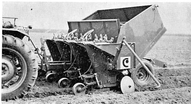
Fig. 2. Automatic planter with big hopper.
