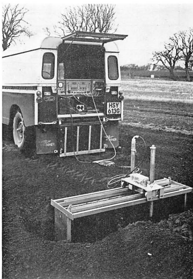
Fig. 7. Gamma-ray transmission equipment developed at NIAE Scottish Station for automatic two-dimensional scanning of field soils.
