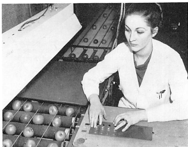
Fig. 7. Apparatus at NIAE for 'keyboard' grading experiments.
