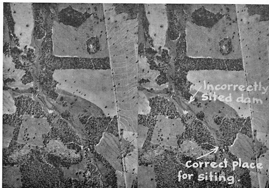
Fig. 11 Training Stereogram showing incorrectly sited existing dam and its correct siting position. Photo Scale 1/20,000
