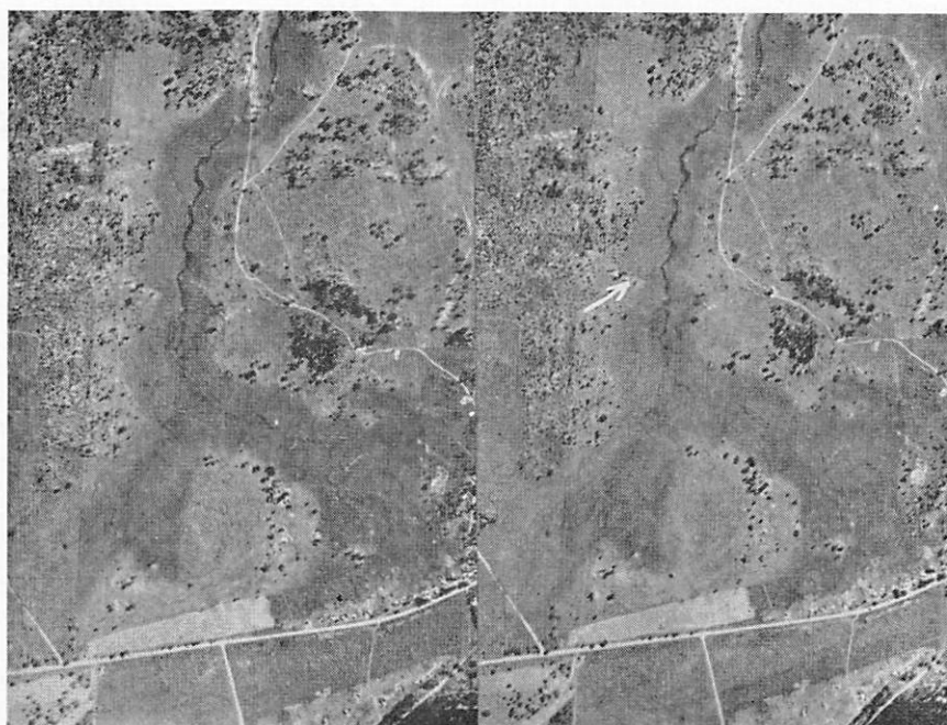
Fig. 10 Stereogram of Dam site. Note rock out- crop at arrowhead—ideal for 'keying in' dam wall. Photo Scale 1/20,000
