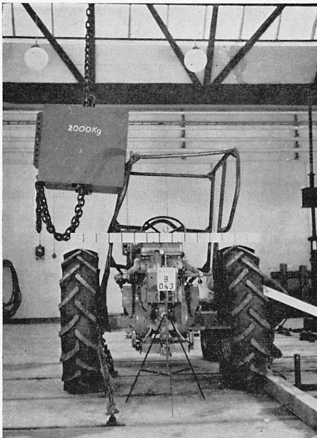
FIG. 3. Impact Test to Side Swedish Testing Station for Agricultural Machinery (Alnarp)
