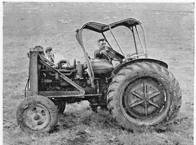
Fig. 8. Safety Frame after eleven sideways and two rearward rolls.
