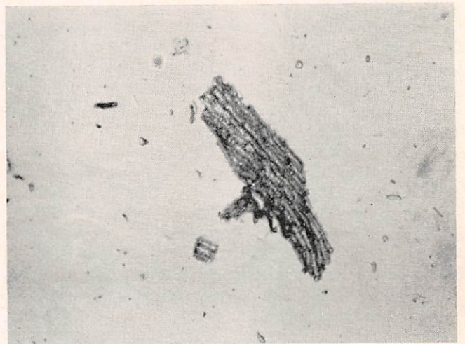
FIG. 8. Siliceous residues—(a) Hay ( \times 42 ), (b) Oat grain ( \times 70 ). (By courtesy of the Journal of Agricultural Engineering Research.)
