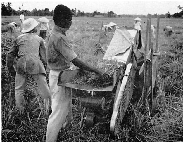
ABOVE: Prototype portable thresher. Trials under local conditions.
