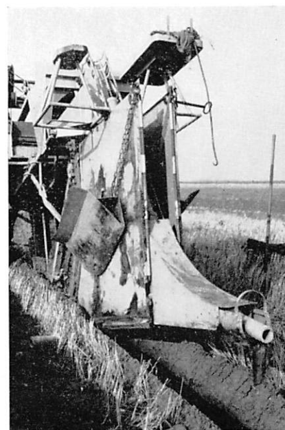
Crumbing shoe and pipe layer of the Buckey drain machine.
