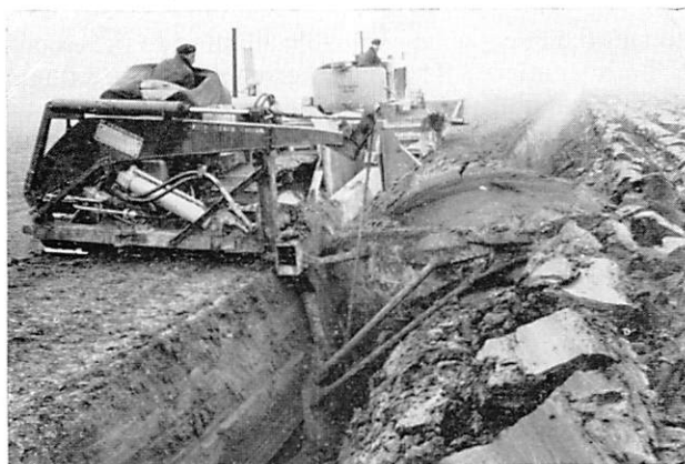
Deep plough. Depth, 1.70 c.m.; the clay is laid on top.
