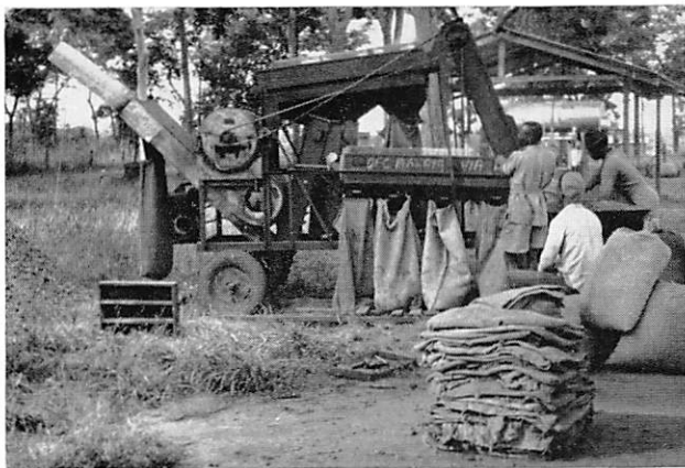
FIG. 5. Groundnut sheller or decorticator and grader.
