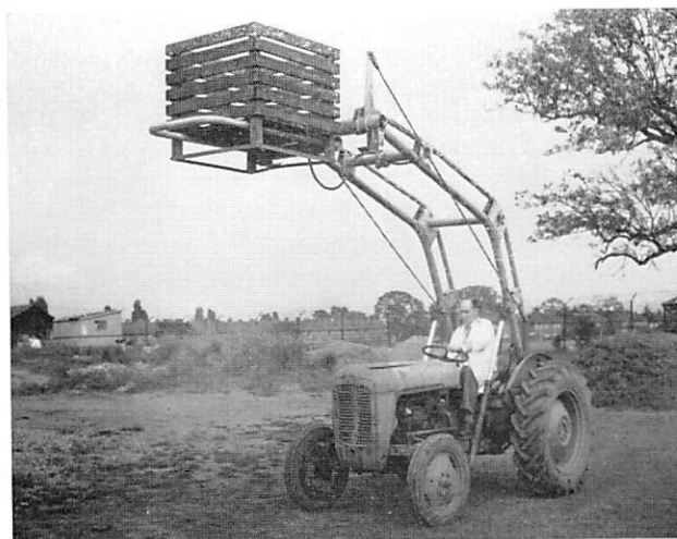
FIG. 3. A side-tipping pallet fork mounted on a tractor front-end loader with parallel linkage attachments. The pallet shown is suitable for handling about 5 cwt. of potatoes.
