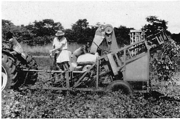
FIG. 6. Complete or once-over groundnut harvester.
