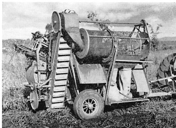
FIG. 12. Cleaning drum for groundnuts on the harvester.
