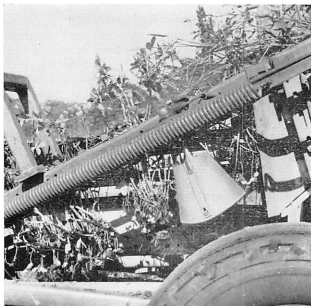
FIG. 10. Agitator for soil removal.
