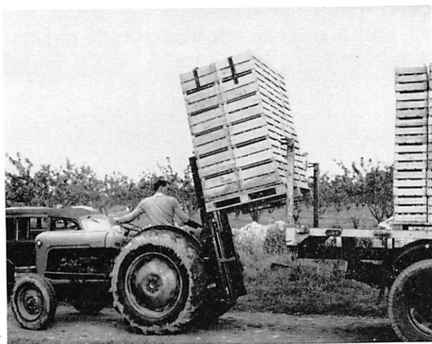
FIG. 2. A low-clearance rear-mounted fork lift of up to 1 ton capacity.
