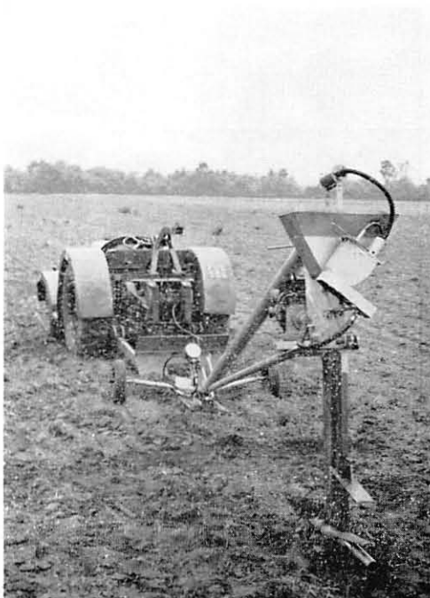
FIG. 4.—Apparatus for Preliminary Installation Tests, fitted with Mechanically-Driven Vibrators.
