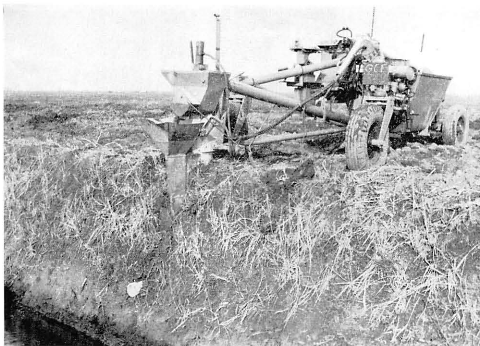
FIG. 10.—Method of Starting from Ditch Side with Pre-fabricated Outfall.
