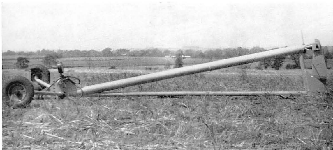
FIG. 2.—Experimental Mole Plough Fitted with Dynamometer.
