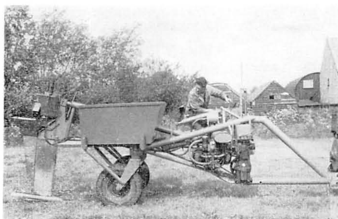
FIG. 7.—The final semi-trailed version of the Vibration Mole Plough.
