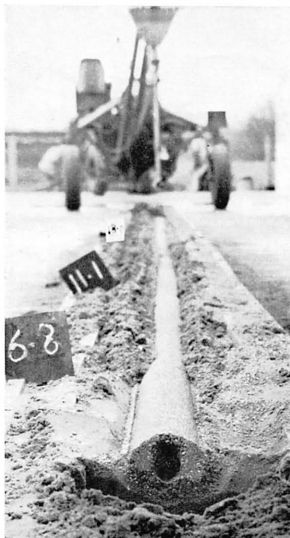
FIG. 9.—Concrete Tube Formed in Testing Tank at Speeds of 6.8 to 18.2-f.p.m.
