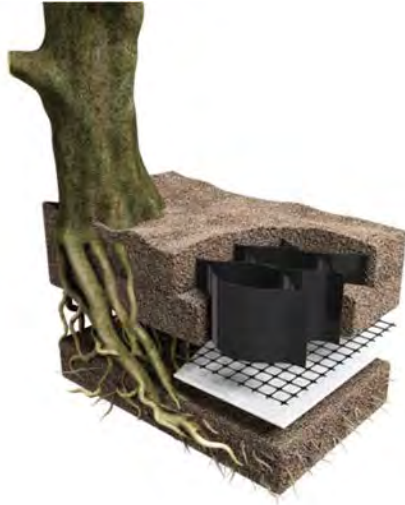
Fig 12 - incorporation of 3D geogrid to achieve BS 5837 compliance
